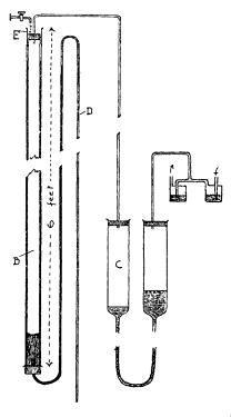
mechanical device of the plunger variety, and the advantages claimed for it are simplicity of construction and perfect continuity of action, once started. Its disadvantages lie in its comparative slowness and its welldefined intermittency. For certain kinds of laboratory work, however, the latter might recommend themselves.
